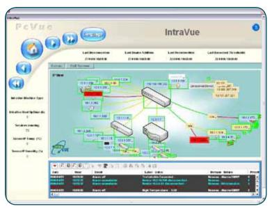
association of the devices with the switches as well as the inter relationships of the networks. The Dashboard is used by Control engineers and Manufacturing IT people.
